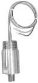
162VTC-XXX-X21-XX With 4-24" flying leads. The dynamic signal leads (black & white) provide a buffered 100 mV/g connection for analysis.
